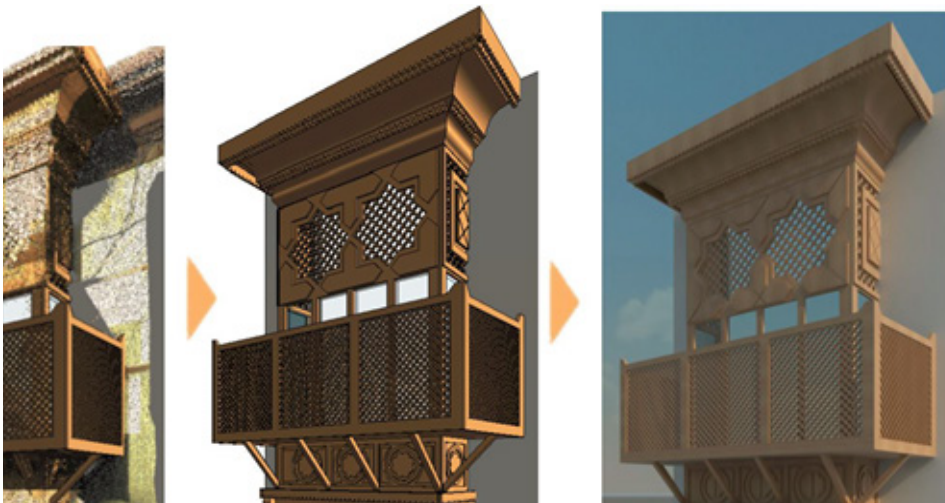
Creation and visualization of a 3D model based on a point cloud
